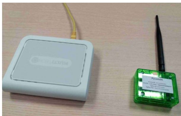
Fig. 7. Indoor gateway used for Measurement 3 experiments on the left side, and packaged Pycom device on the right side.
