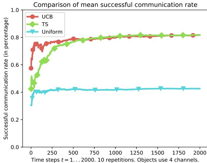
Fig. 4: Less than 400 communication slots (*i.e.*, less than 100 trials in each channel) suffice for the two learning objects to reach a successful communication rate close to 80%, which is **twice as much** as the non-learning (uniform) object, which stays around 40% of success. Similar gains of performance were obtained in many different scenarios.
