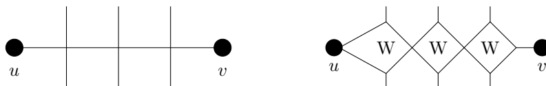
FIGURE 7.11: Elementary step in the transformation of a nonplanar graph into a planar graph. An intersection in the left-hand-side graph is removed by the insertion of a widget (right-hand-side graph).
